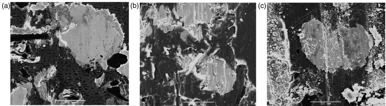
Fig. 11. SEM analysis of bronze and CF filled PTFE composites after tribological tests at (a) RT in air, (b) T=77 K in \text{LN}_2 , (c) T=4.2 K in LHe ( F_N=50 N; v=1.0 m/s; s=2000 m).
